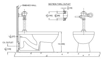
Rough-in/Overview dimensions for Z5635 Series Z5635-BWL with top spud Z5636-BWL with top spud and bedpan lugs
